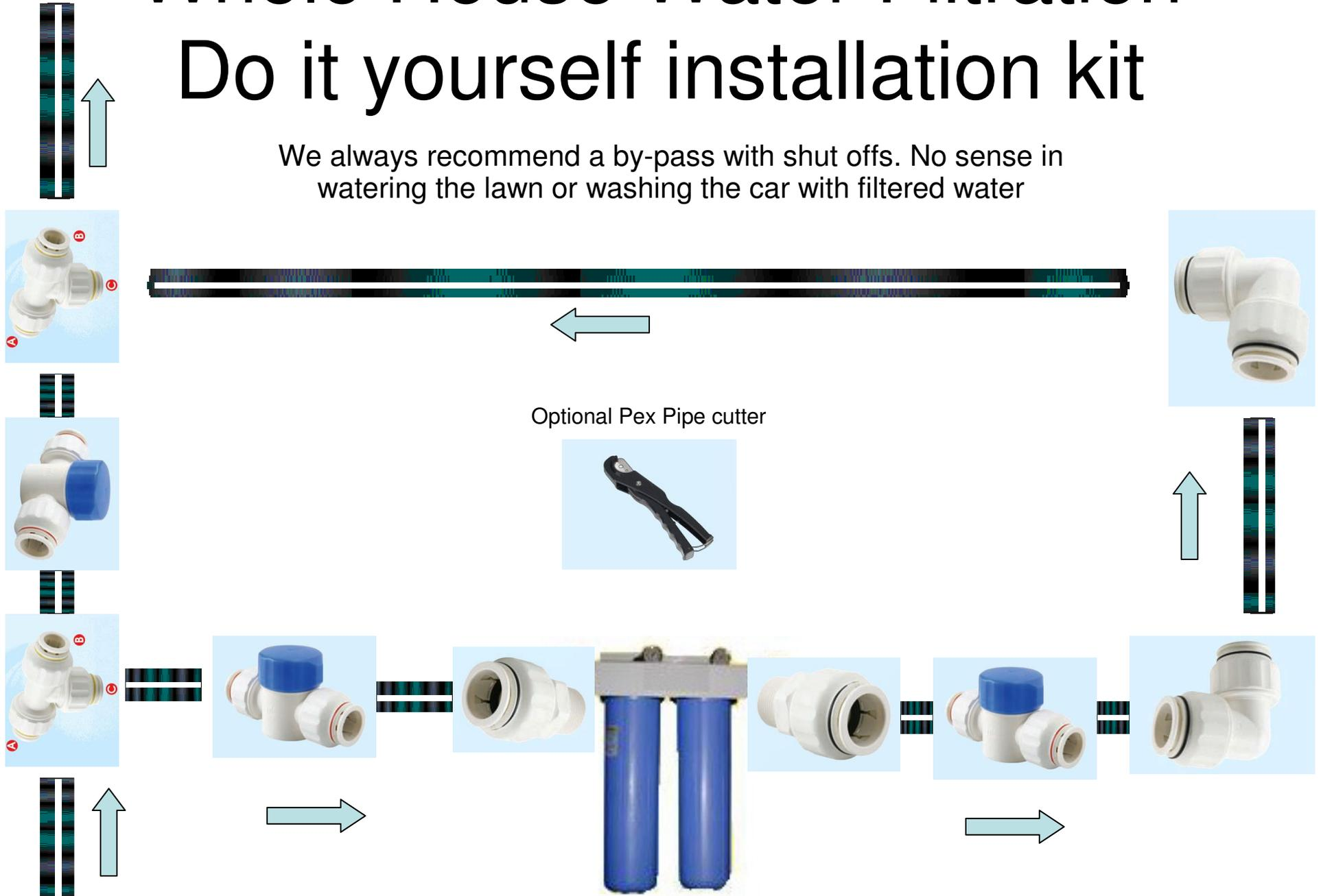
To by-pass the system, simply shut off the two valves on both sides of the housing and open the shut off valve on the left.
